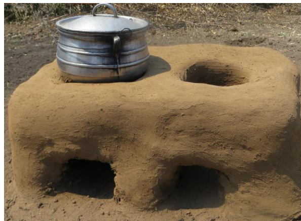
Fig. 13. A fuel efficient stove - Community innovations
