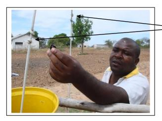
This RWP was installed within the past 4 months and yet it has already lost 25% of its washers! Note the torn washer that was found next to the pump. It is highly unlikely that this pump will still be working at all in a short period of time.... Like most of the others??
