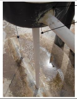
Note the various attempts at Trinipon repairs on this RWP. Such leaks will obviously reduce delivery quite significantly. This poor RWP model was eventually dropped as further refinements were necessarily introduced.
