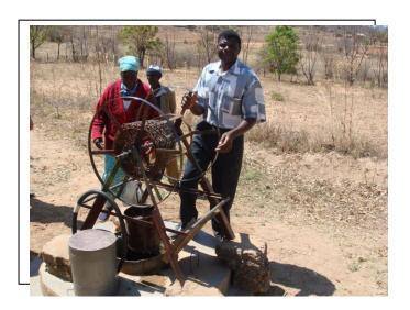
Yet another 'home grown' version of the bucket and windlass water lifting device that has proven to be both robust, and very sustainable.
